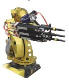
Multi Spindle Robot end effector solution with advanced tightening strategies, error proofing and data collection, reconfigurable for optimum productivity
